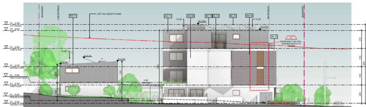
Figure 1: Extract of Architectural Plans showing CBLEP 2023's prescribed maximum Building Height in relation to the proposed development
